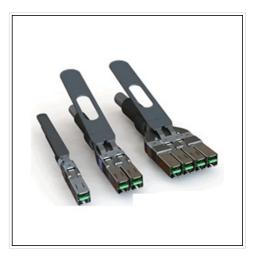
The RCx1 (single-lane) cable design features two differential pairs, four surrounding ground contacts, and two ID pin contacts on a 0.8mm pitch. The RCx2 (dual-lane) and RCx4 (quad-lane) configurations are multiples of the RCx1 configuration. A mechanical keying slot in the center of the bottom of the cable connector shield prevents mismating of the connector orientation, as well as improper lane-shifting errors.
